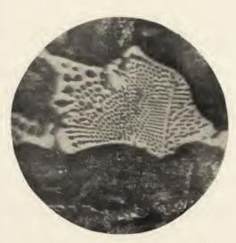
Fig. 25. Highly magnified photograph of one of the phosphide eutectic areas. The ground mass was darkened to show the eutectic structure more clearly.
